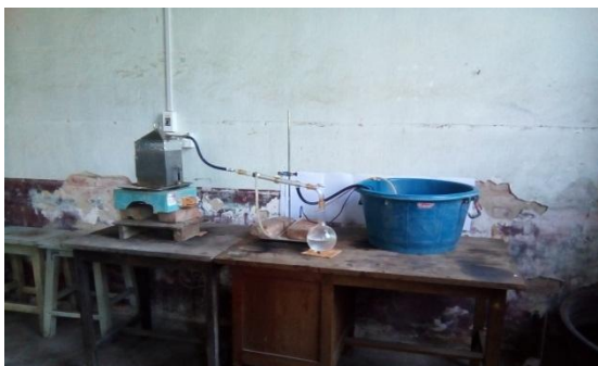
Figure 2: Steam Distillation Apparatus
